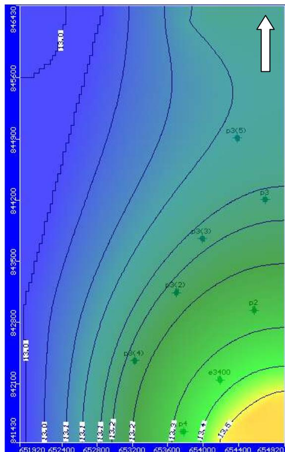
Figure (11): Water level contour map of the unsteady state during year 2040.
