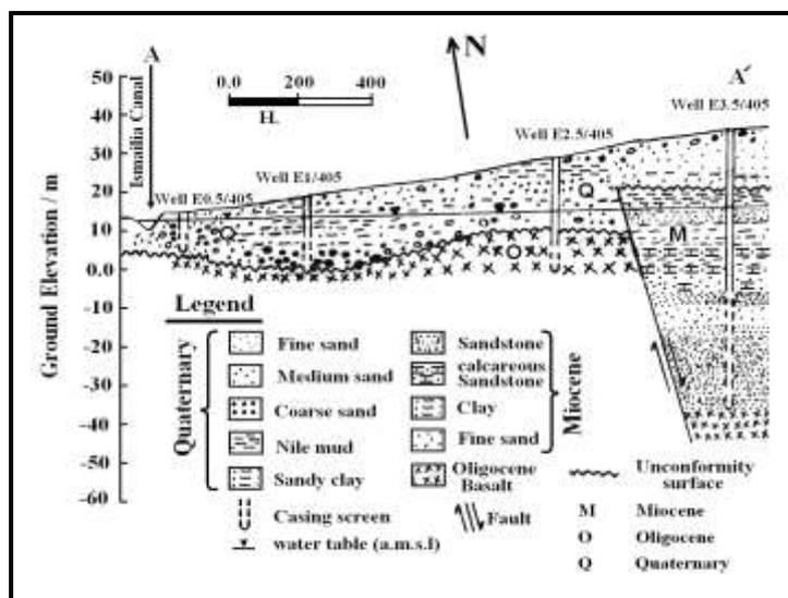
Figure (4a): Geological Cross section ` , EAEA site Inshas area, (Al Gamal et al, 2011).
