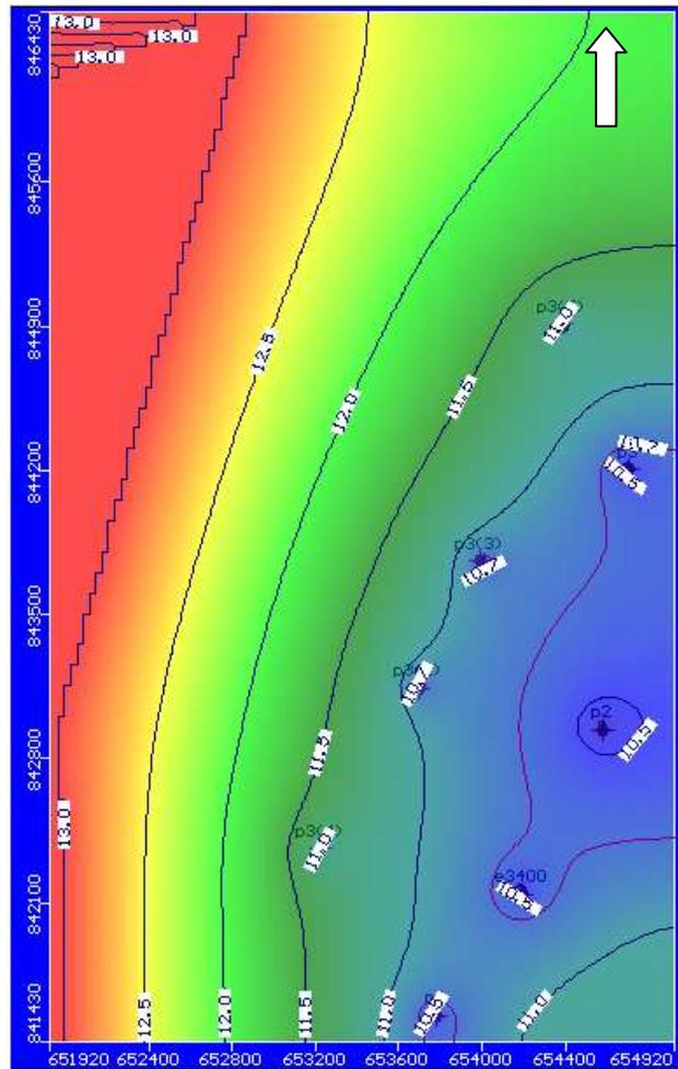
**Figure (14):** The predicted head from 3<sup>rd</sup> scenario in the year 2040.
