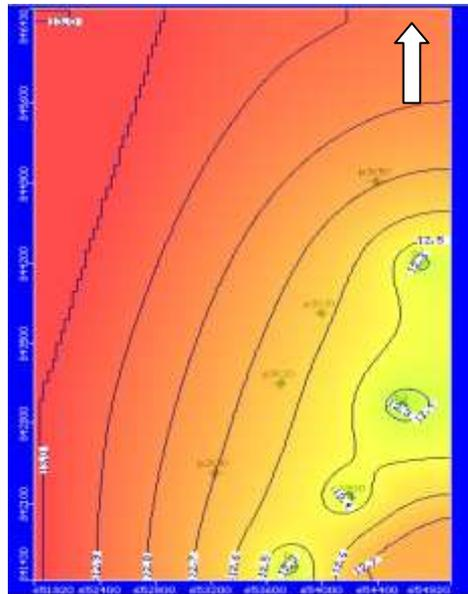
**Figure (12):** The predicted head from 1<sup>st</sup> scenario in the year 2040.
