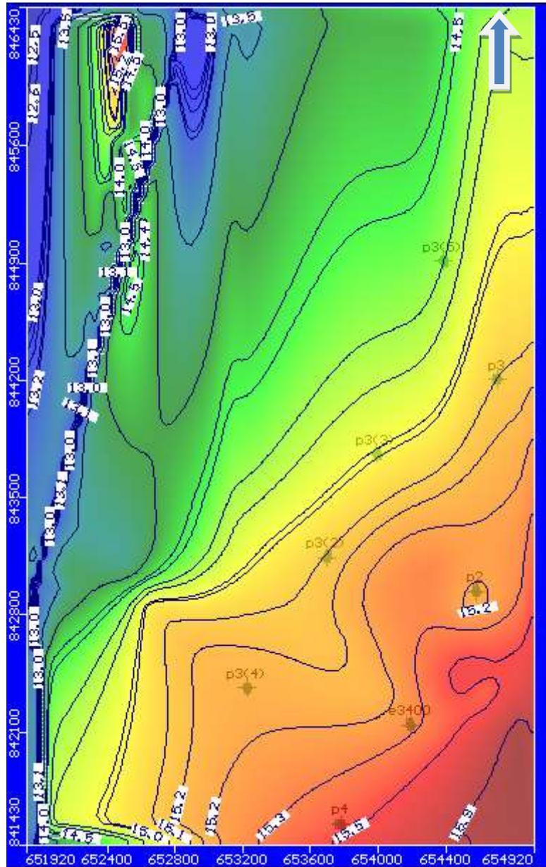
**Figure (9):** Water level contour map of the unsteady state during year 2005.
